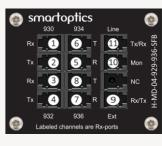
Note row dependent location of Tx and Rx ports. This is due to the usage of duplex LC connectors.
