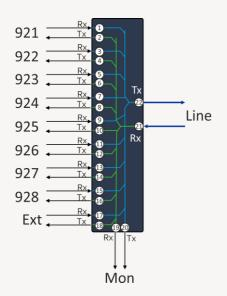
Client and Line signals entering the filter is denoted "Rx". Client and Line signals exiting the filter is denoted "Tx".
