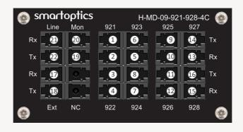
The port allocation and overlay example is for H-MD-09-921-928-4C. Note row dependent location of Tx and Rx ports. This is due to the usage of duplex LC connectors.
