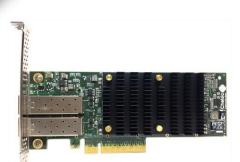
T6225-CR provides sub micro-second end-to-end latency, while offloading the host CPU from a variety of typical storage, networking, and cloud related protocols. This will enable savings in host CPU acquisition costs, power and operational costs, and dramatically increases system performance.
