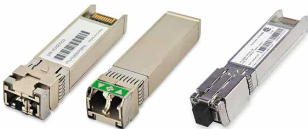
Figure 1: Duplex and bidirectional wavelength-tunable DWDM SFP+ transceivers.
