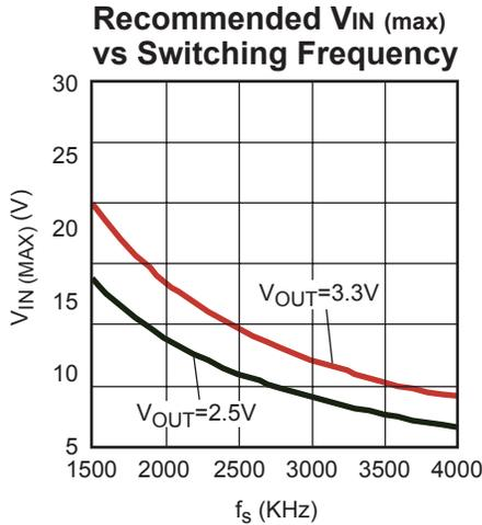
Figure 2—Recommend Max V<sub>IN</sub> vs. f<sub>s</sub>
