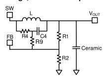
Figure 11: Simplified Ceramic Capacitor Circuit
