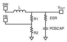
Figure 6: Simplified PWM-Mode Circuit without External Ramp Compensation
