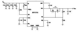
Figure 13: Schematic Reference for PCB Layout
