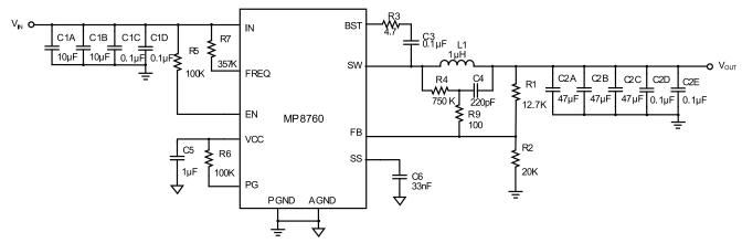
Figure 16—Typical Application Circuit with Low ESR Ceramic Capacitor for 1V Output
