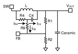
Figure 7: Simplified PWM-Mode Circuit with External Ramp Compensation
