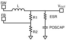
Figure 10: Simplified POSCAP Circuit
