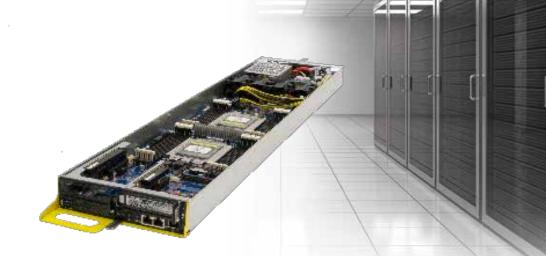
Penguin Computing Altus X01132g is an Open Compute Server, and part of the Penguin Computing Tundra Extreme Scale (ES) Family. Featuring a 10U 3 Node server powered by AMD® EPYC® Processor, it is a high density server targeting high performance computing and highly optimized for hyper-scale deployment. Altus X01132g supports up to 128 PCle Gen3 lanes, with capability to handle multiple NVMe devices and OCP Mezz card options.
